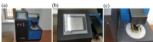
Fig. 3: Photos of the tag closed cup tester: a) Whole apparatus; b) Control panel and c) Gauge
