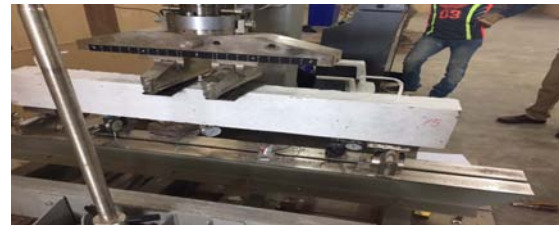
Fig. 3: Testing machine of RC beams
