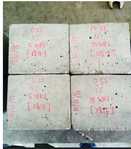
Fig. 4: Concrete cube specimen
