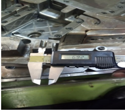
Fig. 3: Gate size: 6.92 mm
