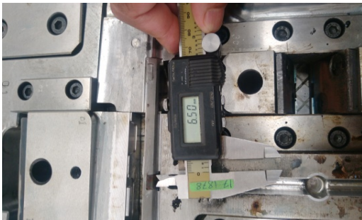
Fig. 2: Gate size 6.5 mm
