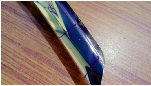
Fig. 1: Silver streaks on plated part
