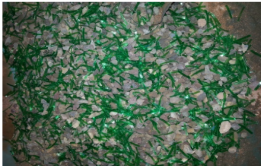
Fig. 4: The dry ingredients with waste plastic fibers
