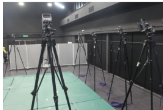
Fig. 16: 12 motion capture camera on stage
