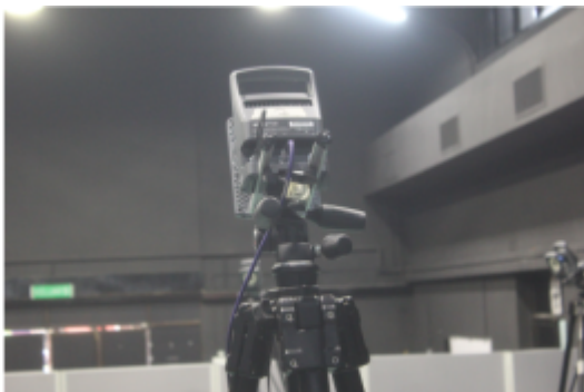
Fig. 15: Motion capture camera
