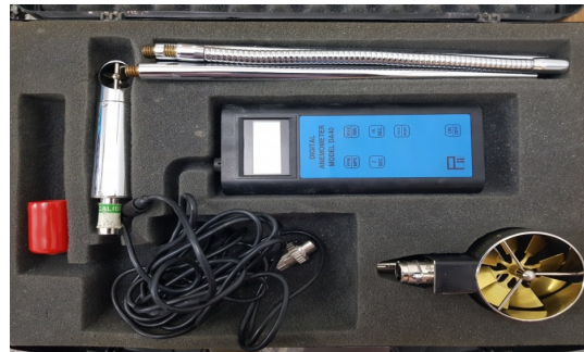
Fig. 5: The digital air anemometer
