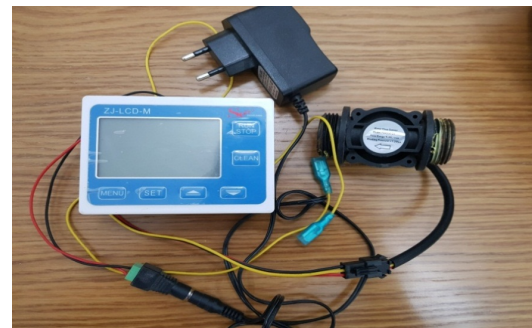
Fig. 6: The digital water flow meter used to measure the water flow rate between cooling tower and heat exchanger
