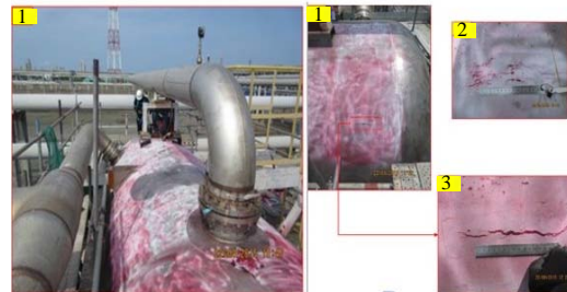
Fig. 6: Crack found at internal top tank same location as the external surface
