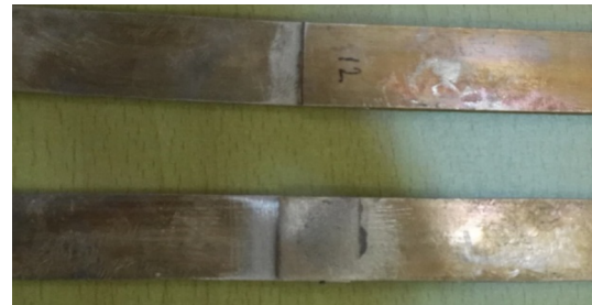
Fig. 3: Copper adherents after pressing
