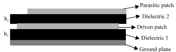
Fig. 3: Side view of proposed stacked antenna
