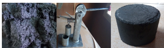
Fig. 4: Biofuel formulation process
