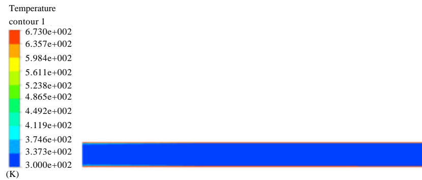
Fig. 4: Temperature distribution for smooth elliptical passage
