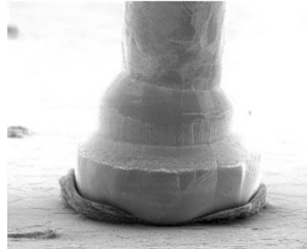
Fig. 13: Bond on high thickness Al bond pad
