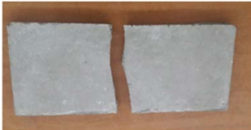
Fig. 7: Cementitious board: a) Self-curing specimens before test and b) After bending test
