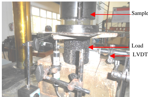
Fig. 4: Setup for the compressive strength test
