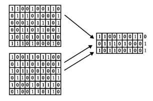
Fig. 3: A crossover process: a) Solution A; b) Solution B and c) Solution C
