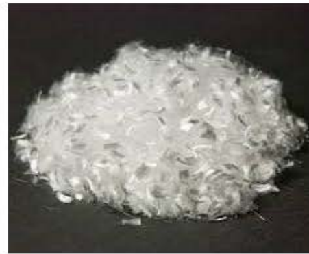
Fig. 2: Fibrillated polypropylene fibers used in present work
