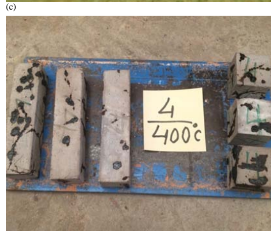
Fig. 8: a) Mortars samples with 0.5% WPF after exposure to 400°C temperature; b) 1% and c) 1.5%
