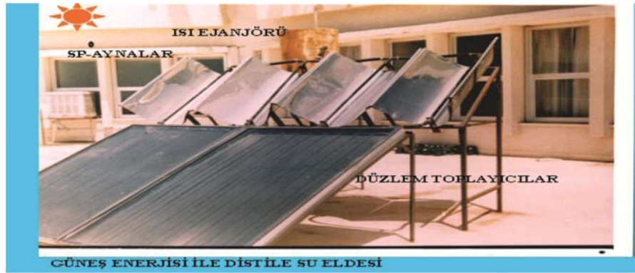
Fig. 3: The plane collector and cylinder parabolic concentrators together with heat exchanger in a water distillation system (Arslan and Aydinol, 2011)
