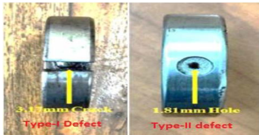
Fig. 5: The type-1 and 2 defect bearing
