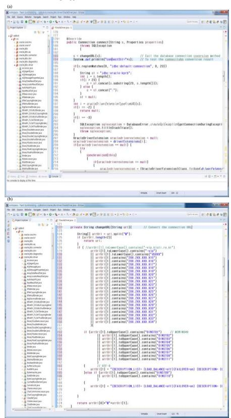
Fig. 1: a, b) Implementation of database connection URL conversion function
