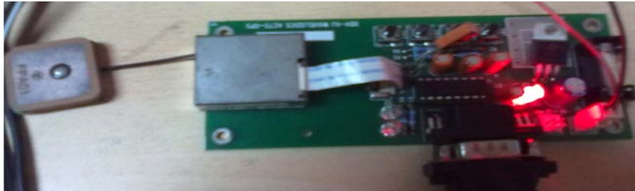
Fig. 12: Interfacing of serial to USB converter
