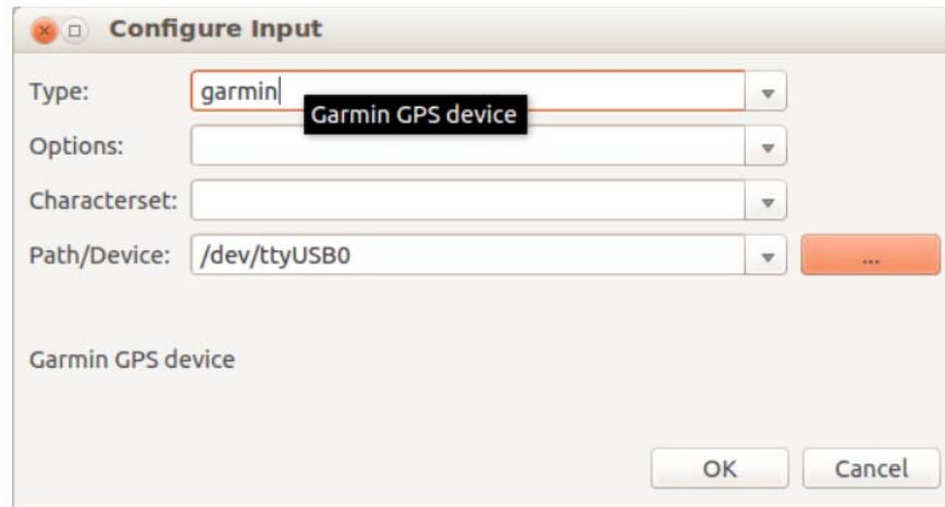
Fig. 10: USB Garmin GPS device setup
