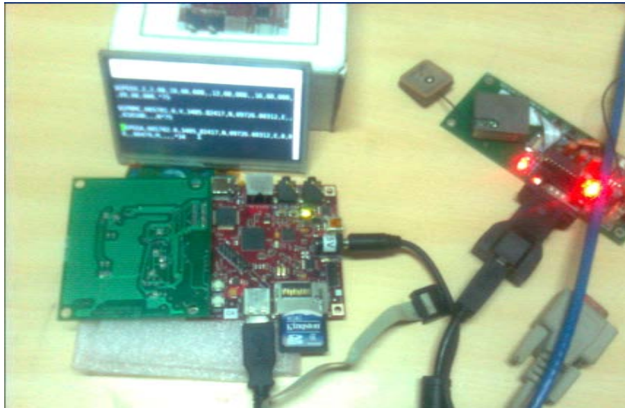
Fig. 13: GPS receiver interfacing with Beagle board
