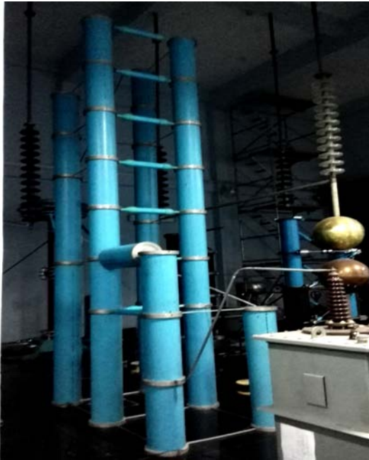
Fig. 4: Cockcroft-Walton circuit DC generator 0-100 kV
