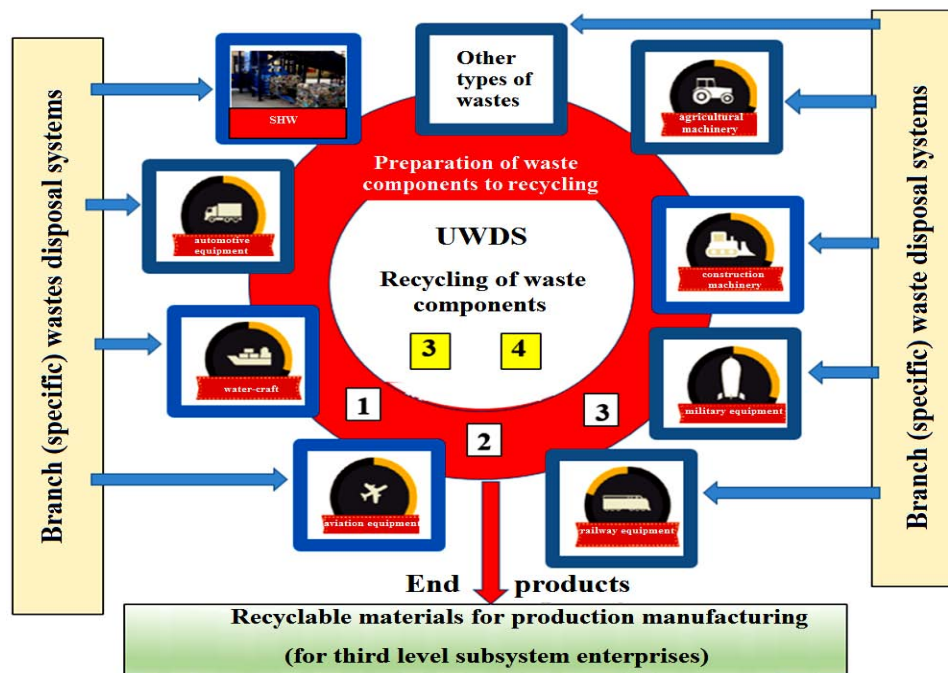
Fig. 5: Unified wastes disposal system structure
