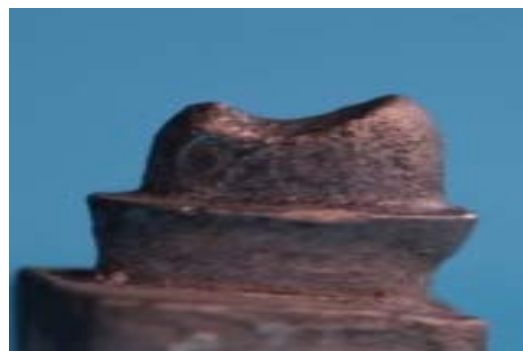
Fig. 1: Master metal die with 8° taper
