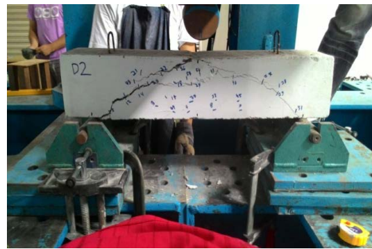
Fig. 8: Mode of failure for retrofitted sample
