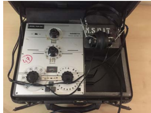
Fig. 1: PAM 010 audiometer unit used to measure the hearing threshold
