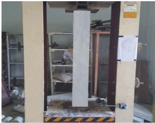
Fig. 2: Reference column in testing machine
