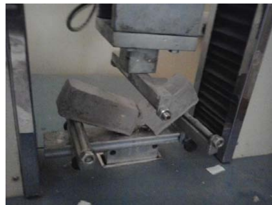
Fig. 4: Flexural sample at failure
