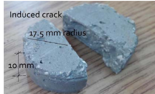
Fig. 5: Water flow sample broken into two pieces
