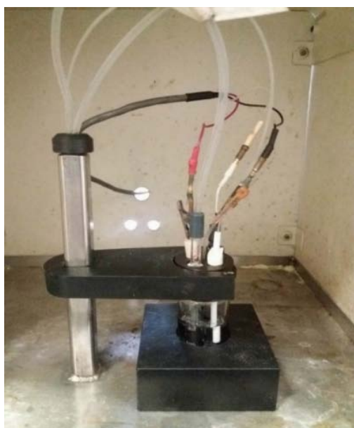
Fig. 2: Mounting of cell for polarization resistance test
