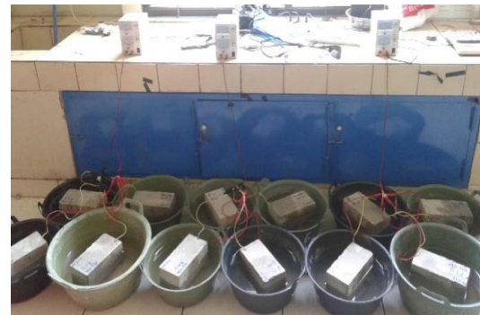
Fig. 2: Accelerated corrosion in laboratory
