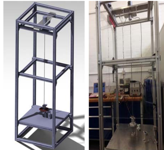
Fig. 1: Laboratory experimental setup (right) drill string experiment; Catia V5 (left)
