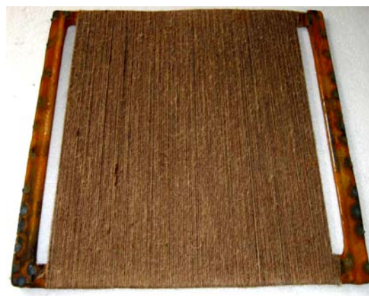
Fig. 1: Four layers of kenaf fiber woven around a steel frame
