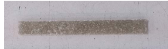
Fig. 4: A composite specimen for flexural bending test
