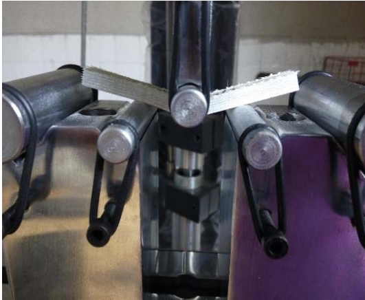
Fig. 9: Nanocomposite under the flexural bending test
