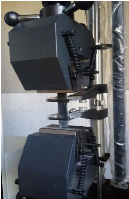
Fig. 6: Clay/nanocomposite during the tensile test
