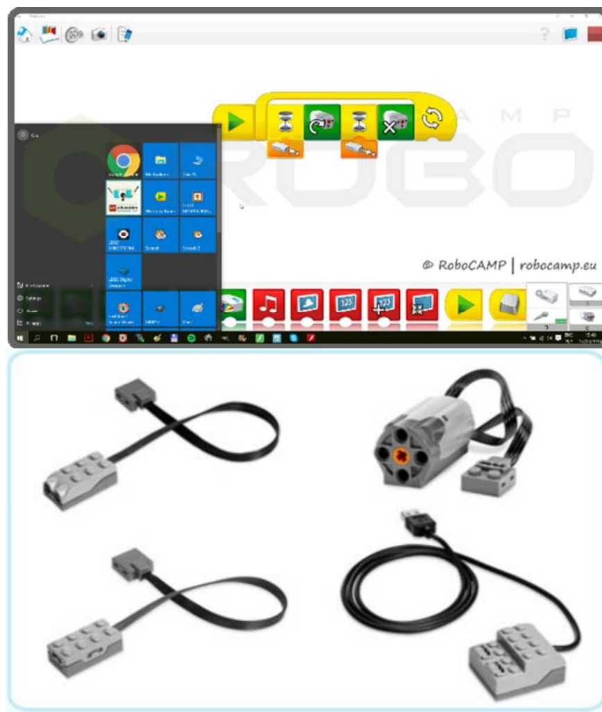
Fig. 1: The WeDo Software interface and WeDo sensors
