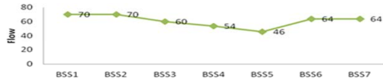
Fig. 7: Flow result for Bitumen-SBS-sulphur mixtures
