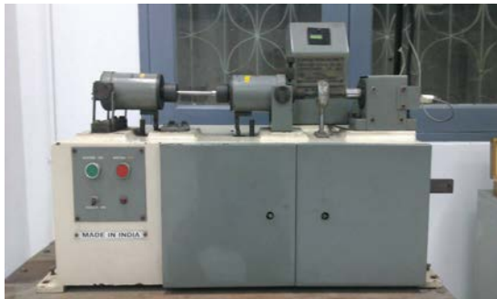
Fig. 10: Fatigue strength testing machine
