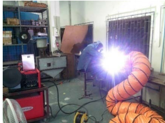
Fig. 5: MIG-MAG welding process with flux-cored wires
