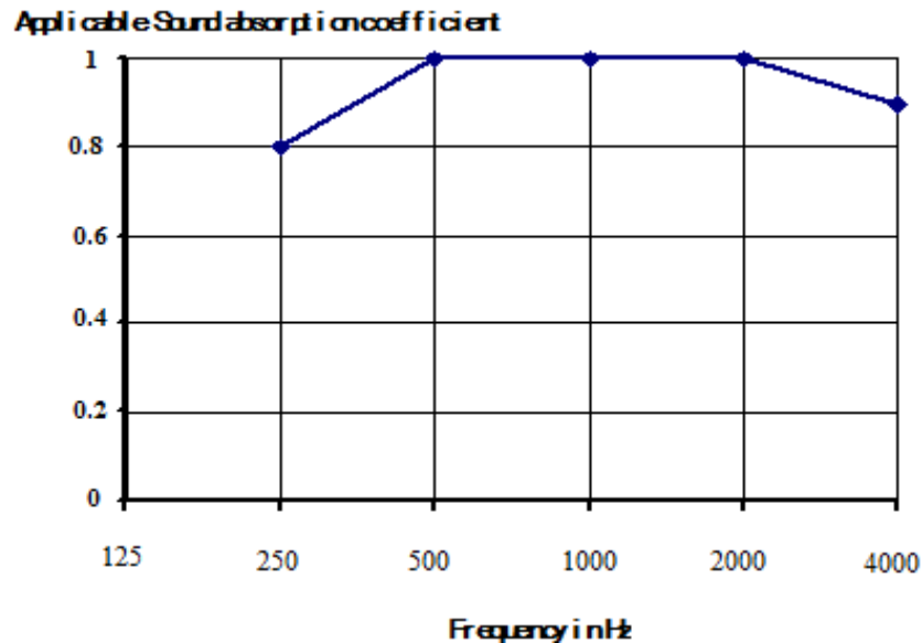
Fig. 5: Reference diagram for evaluation of weighted sound absorption coefficient of \alpha_w
