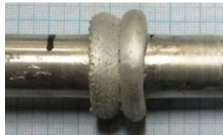
Fig. 4: Chamfer angle of 0^\circ , surface roughness of 0.697 \mu\text{m}
