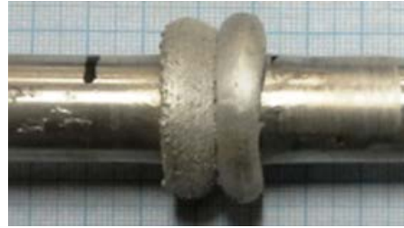
Fig. 3: Without chamfer angle ( 0^\circ ), surface roughness of 1.0667 \mu\text{m}
