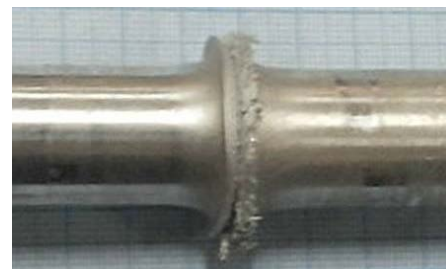
Fig. 6: Chamfer angle of 15^\circ , surface roughness of 0.697 \mu\text{m}
