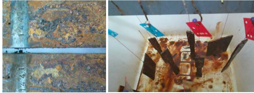
Fig. 2: Corroded plates in salt spray machine
