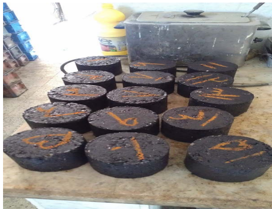
Fig. 9: Samples came out of asphalt bathroom
