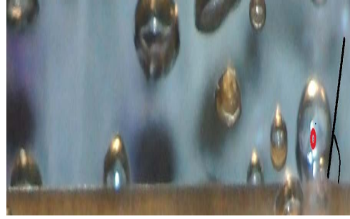
Fig. 4: The dynamic contact angle on the Aluminum surface
