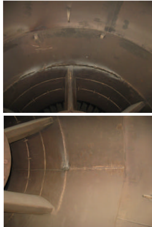
Fig. 1: A view from inside of the diffuser examined and location of the temperature sensor and repaired welds
