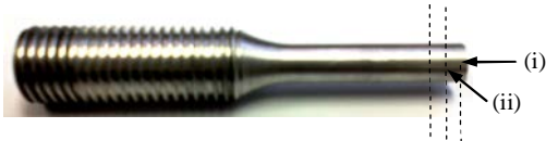
Fig. 5: Fatigue fracture surface indicates by (i) and the hardness test was performed about mm under the fracture surface as indicated by (ii)
