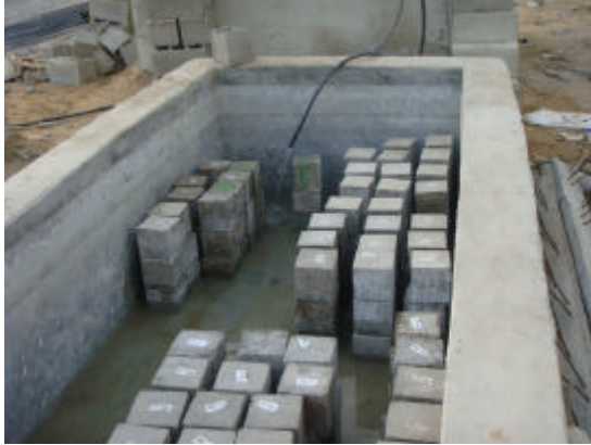
Fig. 4: Curing samples in a tidal environment
