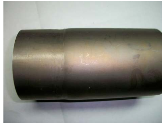
Fig. 2: A thin-walled precision pipe with a diameter D = 80 mm with wall thickness t = 0.8 mm from PT-7M titanium alloy with calibrated end by the squeezing mode
