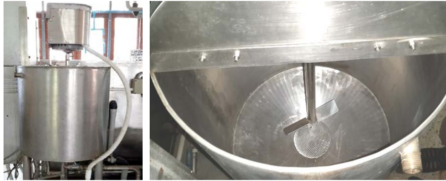
Fig. 3: Inner mixing tank with a paddle
