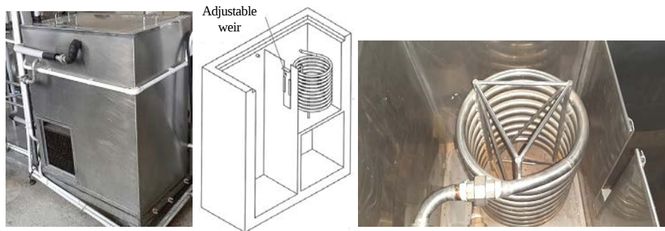
Fig. 5: Cooling tank with inner spiral tube (Jitjaroen et al. , 2008)
