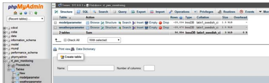
Fig. 5: Two tables of MySQL database in phpMyAdmin tool; WeatherParameter and ModelParameter
