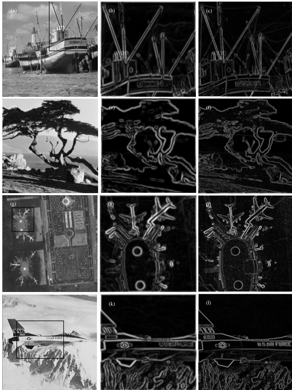
Fig. 2: The localization effect of Gaussian and hyperbolic filtering; a, d, g, j) Original images with cropped area (shown as square box); b, e, h, k) Steerable Gaussian filter responses for variance \sigma = 2 ; c, f, i, l) Steerable hyperbolic filter responses for variance \sigma = 2
