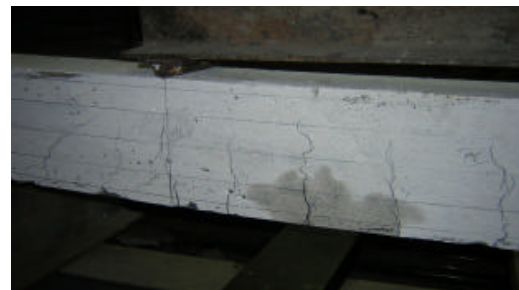
Fig. 5: Failure pattern of the GFRP beam
